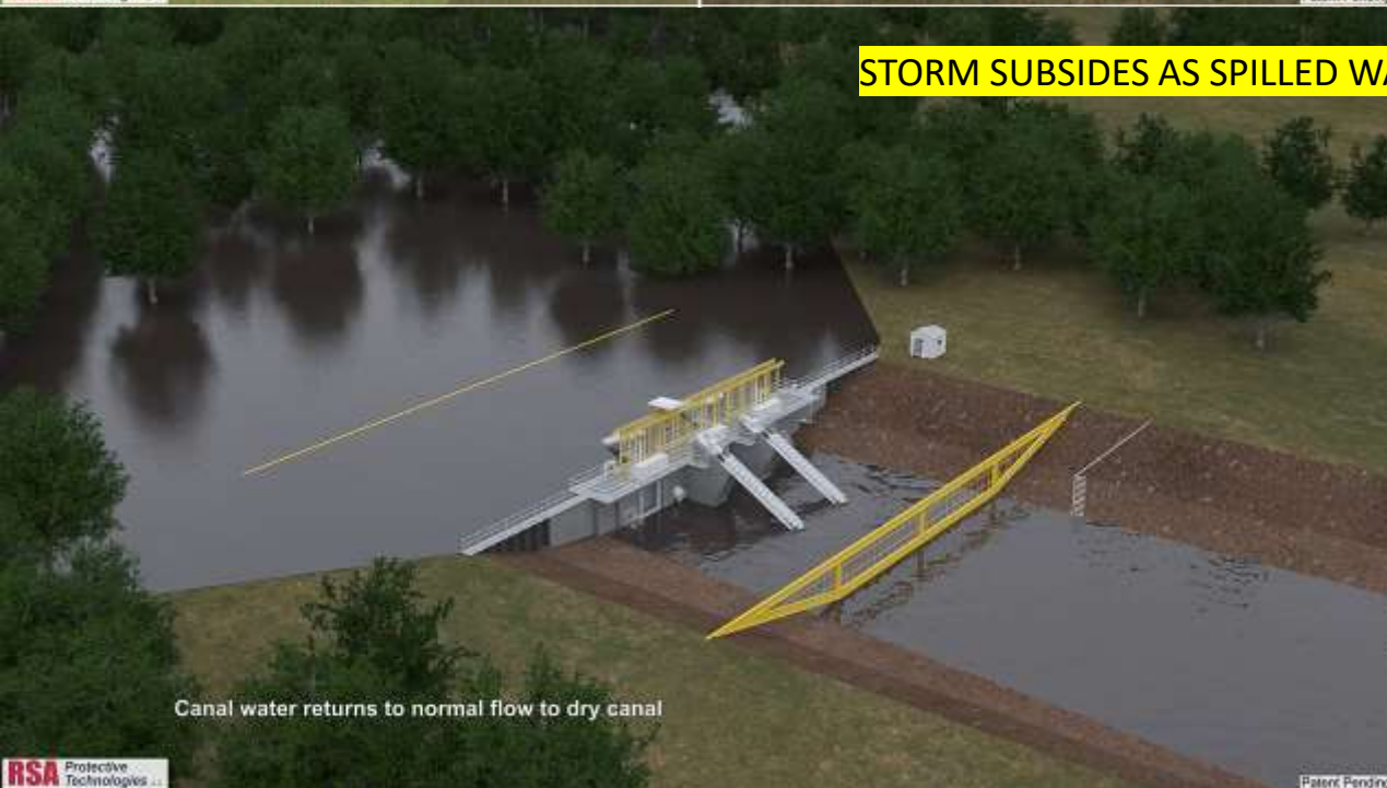
Flooding Open Field lowers Surface Water in canal
