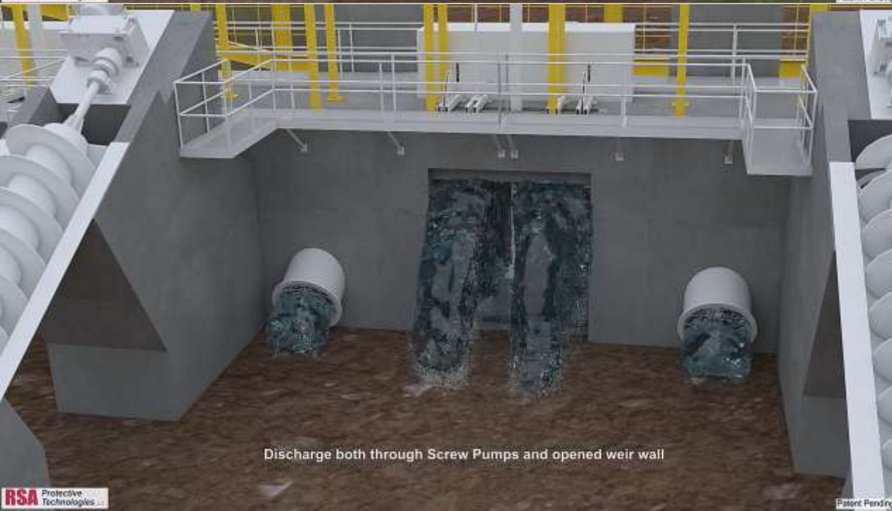
Discharge Screw Pumps drain flooded water from Open Field
