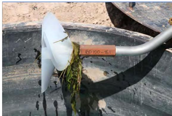
Figure 3. Moss and weed vegetation that fouled the unmodified reverse propeller metering system.
