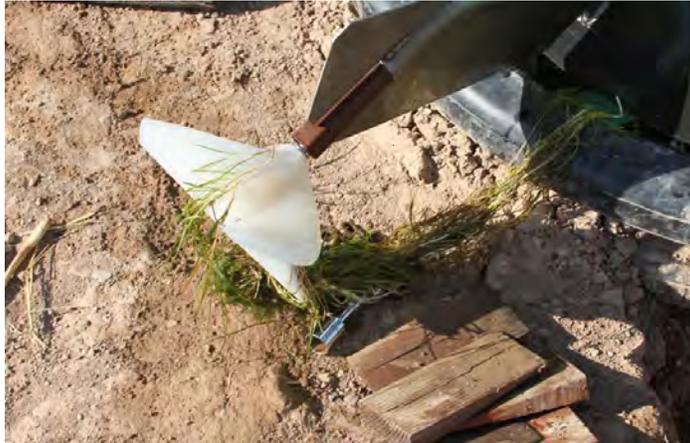
Figure 7. Vegetation is not wound onto meter shaft, so likely was suspended in pipe at shut-off and caught at meter removal. (September 8, 2011).
