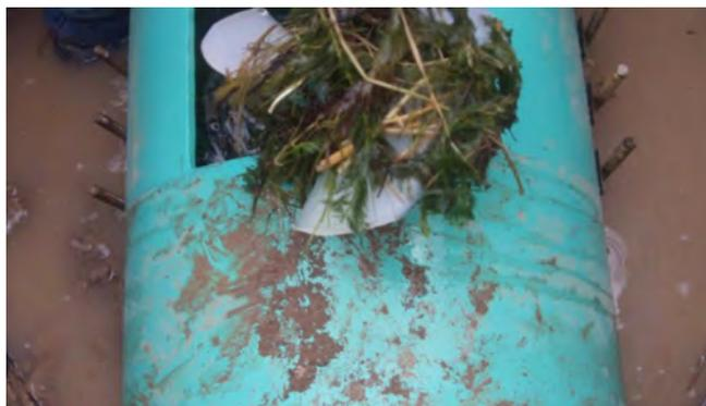
Figure 4. Confirming that the unmodified reverse propeller metering system again clogged.
